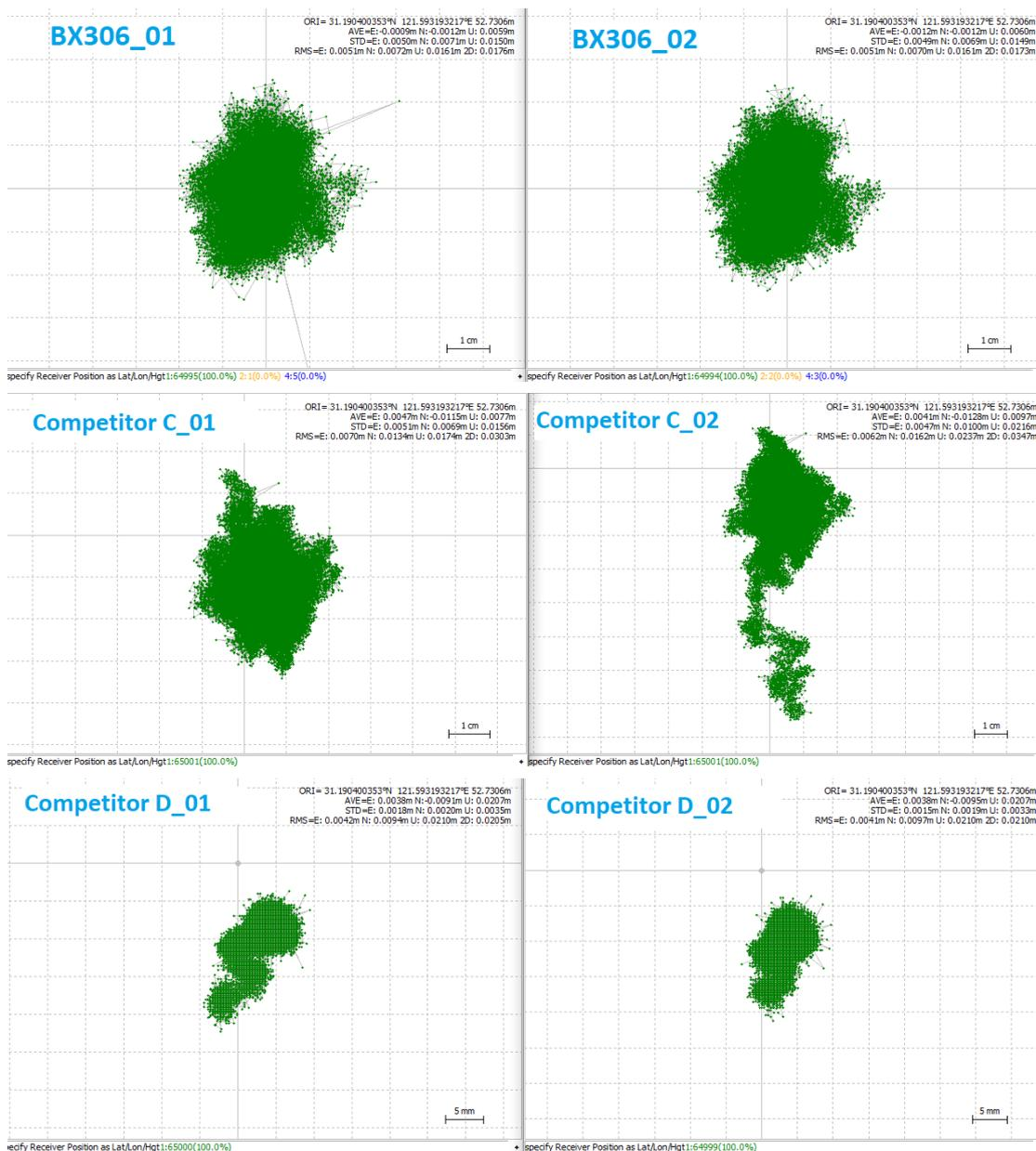
Figure 10 Trajectories of Each OEM boards
