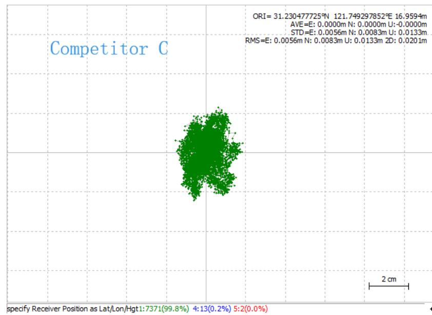
Figure 14 Trajectories of Each OEM boards
