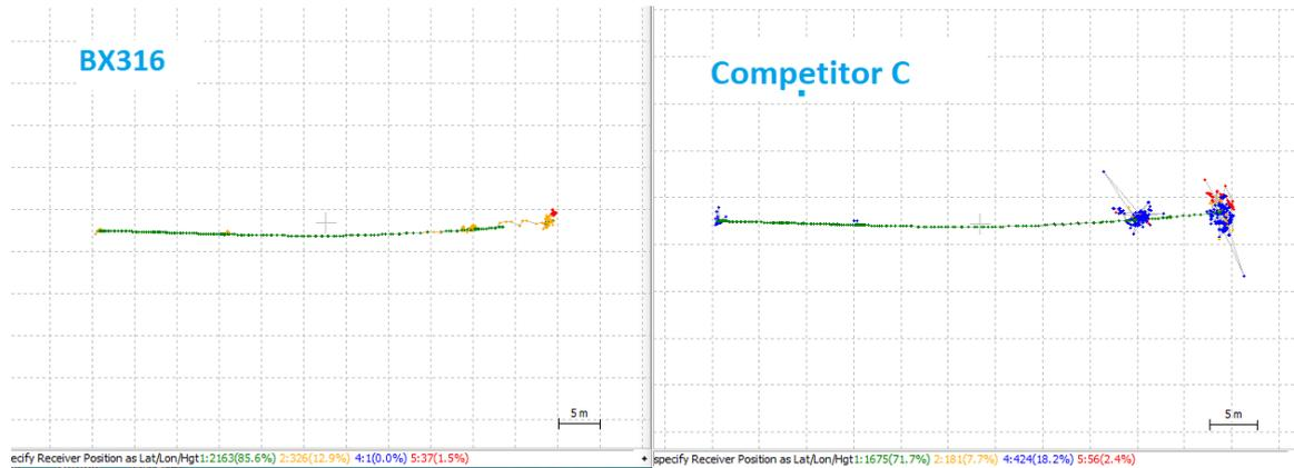
Figure 8 Trajectories of Each OEM boards (dynamic)
