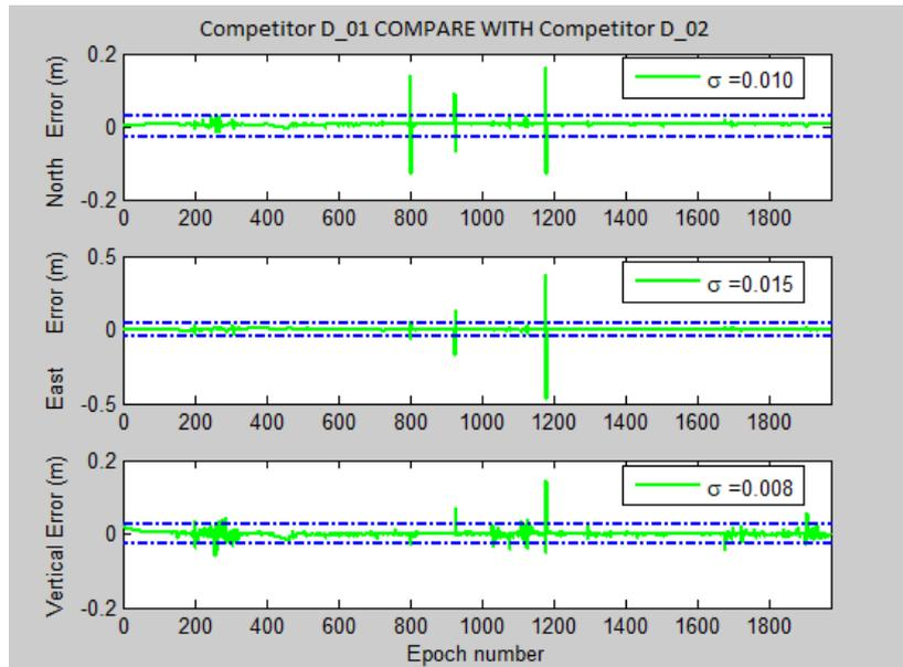
Figure 3 Position Error Time Sequence Diagrams
