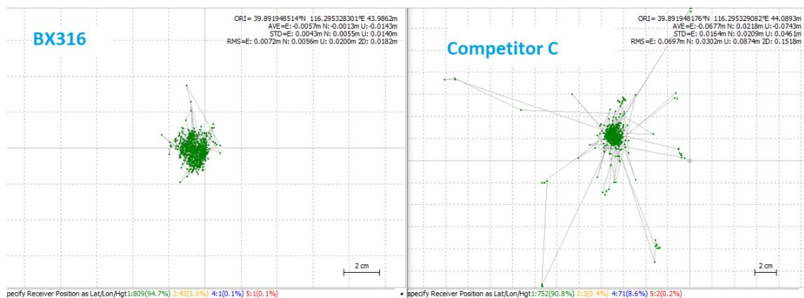
Figure 9 Trajectories of Each OEM boards (static)
